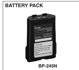
BP-245N Li-Ion BATTERY PACK 7.4V, 1900mAh (min.), 2000mAh (typ.). Provides 15–16 hours* operating time (approx.). Same as supplied. *(Tx (Hi): Rx: standby=5:5:90).
