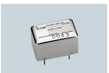
CR-338 HIGH STABILITY CRYSTAL UNIT Contains a temp. compensating heater for improved frequency stability. Frequency stability: ±0.5 ppm
